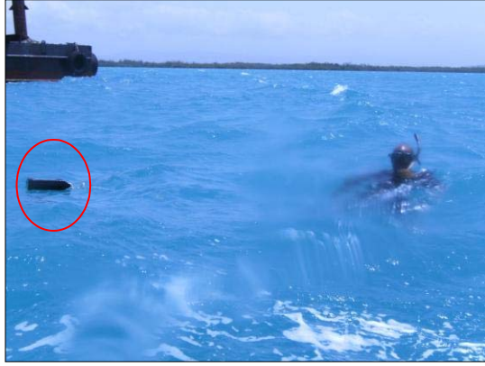
Figure 3: Photo showing marker buoy (indicated by red circle) above the C1 borehole in front of the barge; (Photo taken -15 August 2014)
